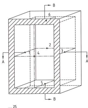
Thermocouple 1-6 Location: Inside the cabinet, 25mm from the surface
